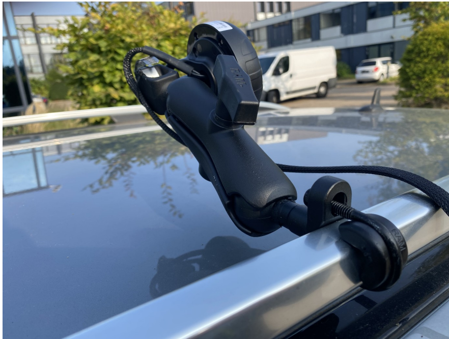
Fig. 11: Assembly MRX.planarAntenna with magnetic base
