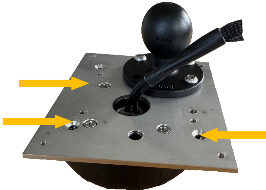
Fig. 10: Mounting MRX.planarAntenna to MRX.mountingPlate
