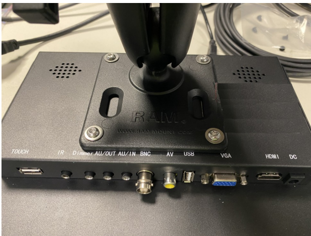
Fig. 4: Mounting VESA on MRX.monitor
