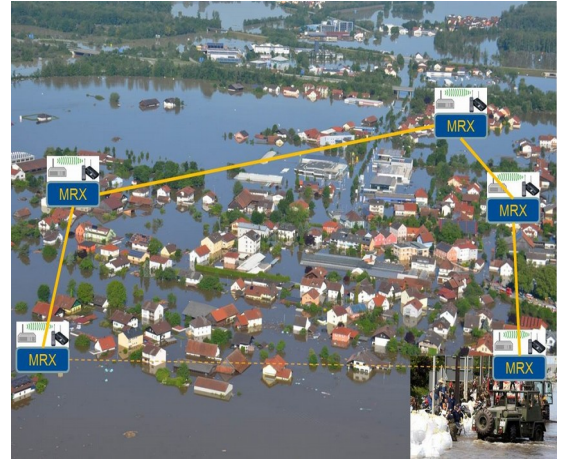
Figure 1: A Mesh network in a disaster area enables voice, video, messaging and other forms of communication if everything else has failed. Battery-powered mesh nodes can be installed on rescue vehicles, or be placed by rescue forces or drones.
