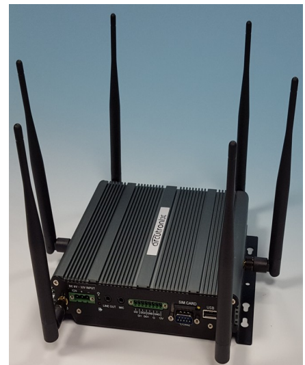
Figure 4: Robust, DC powered Mesh Router with 3 Mesh antennas and 3 WIFI-AP antennas.
